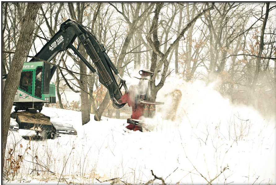
Photo 7: Feller-Buncher Removing Cottonwoods and Ash from Globally Imperiled Ridge & Swale, AER
