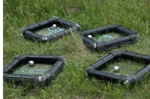
Photo 2 PVC Platform without Foam or Carpet Base and with Metal Chain and Lead Fishing Sink
