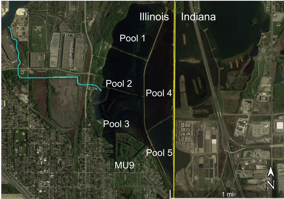
Figure 1. Satellite image of Wolf Lake showing Illinois' five separate pools and the Illinois-Indiana state border in yellow. The pools are separated from each other by berms, but all are hydrologically connected by openings through the berms to allow drainage from pool to pool and eventually to the Calumet River (upper left) via Indian Creek (in blue). Imagery courtesy of Google Earth.
