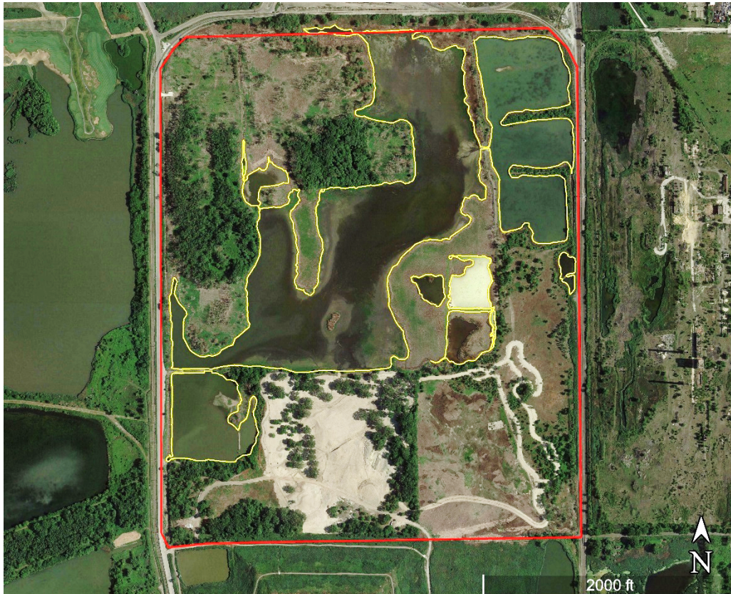
Figure 1. A 2016 satellite image of the 300-acre Big Marsh site owned by the Chicago Park District outlined in green. Pools comprising 96 acres of water are outlined in yellow. All areas not outlined in yellow were created by the deposition of slag or other material into the Calumet marshes. Imagery courtesy of Google Earth.
