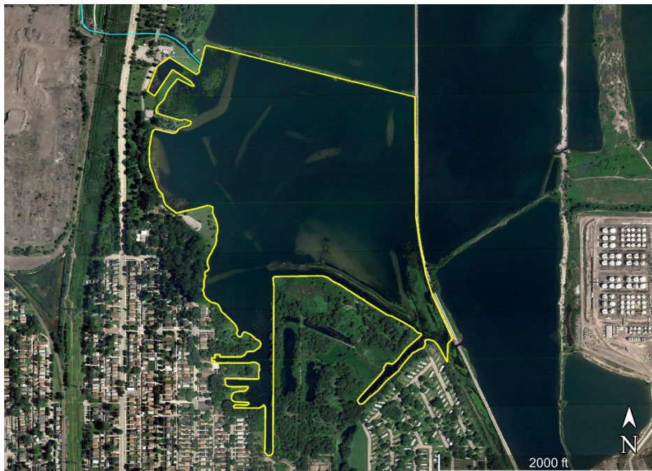
Figure 2. Wolf Lake's Pool 3, outlined in yellow, with the outlet stream at Indian Creek designated by the blue line. Pool 3 is separated from Pool 2 to the north by a berm, and from Pools 4 and 5 to the east by a berm and rail line. Imagery courtesy of Google Earth.
