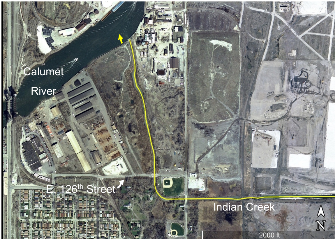
Figure 2. A 2002 satellite image showing the flow path of Indian Creek (in yellow) prior to riparian restoration in 2003. The creek channel north of E. 126th Street was meandered to create a longer reach and an extended riparian wetland along its length. Image courtesy of Google Earth.
