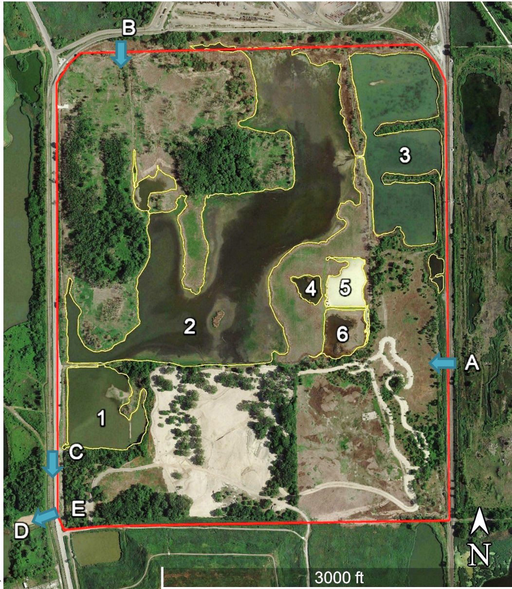
Figure 4. Hydrologic characteristics of Big Marsh, with major pools (1 through 6), inlets (A, B, and F), water control structures (C and D), and the dam created by the new entryway culverts (E). Imagery courtesy of Google Earth.
